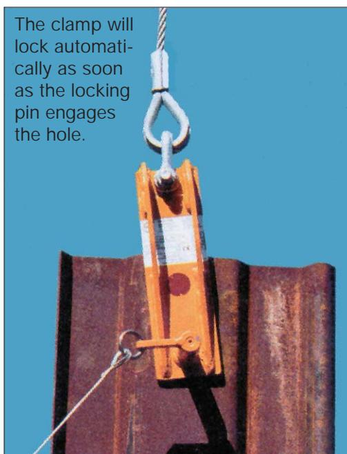
The clamp will lock automatically as soon as the locking pin engages the hole.
