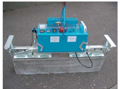
Carrying module G 5 with 2 adjustable suction pads, carrying capacity 150 kg *.
